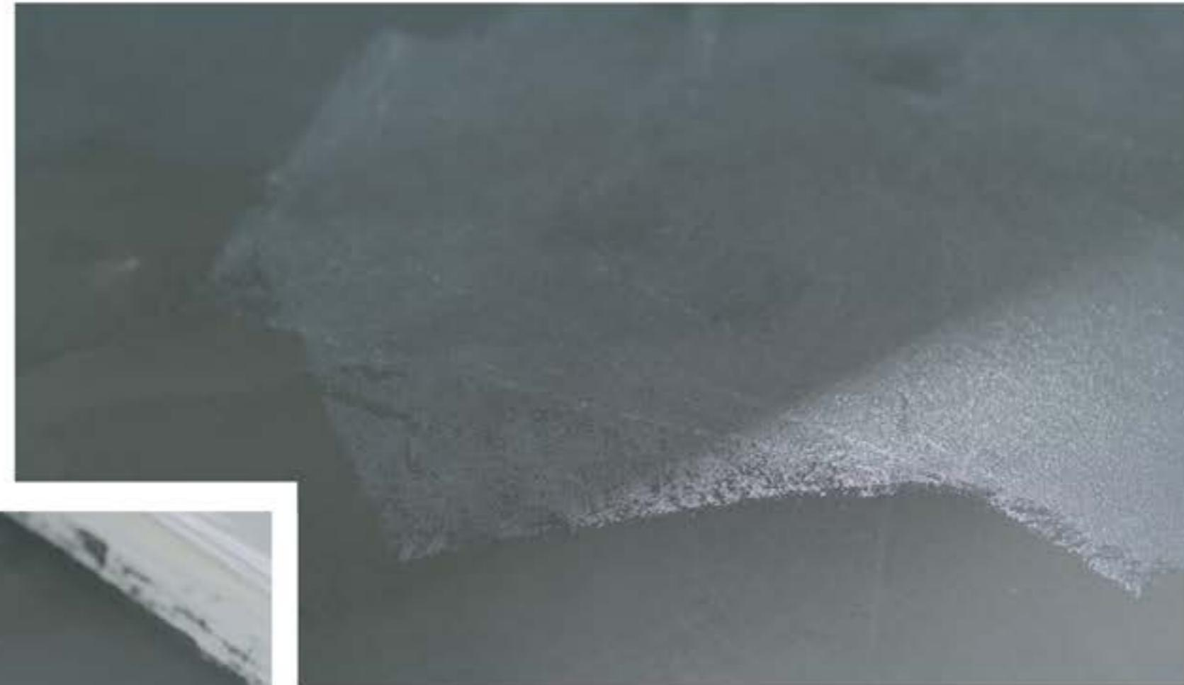
When mixed with water and applied correctly, it fills micropores and creates a barrier that reduces to a minimum humidity absorption from the substrate.
